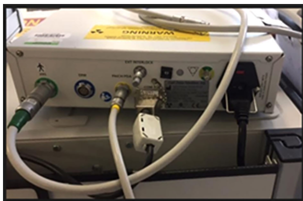
FIGURE A1-1 (a) Connection of x-ray source and photo diode array (PDA) power cables. (b) X-block and x-ray source on rail alignment guide.
